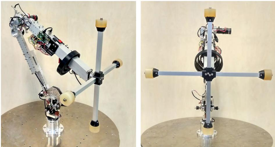
Figure 5.1: Photos of Tippy. The right photo shows Tippy's frontal plane, in which it resembles an RWP.
