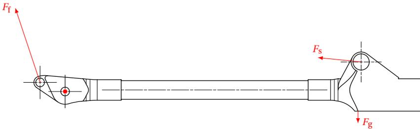
Figure 6.11: Free body diagram of the torso depicting forces as implemented in an FEA. The forces correspond approximately to those of Skippy close to its nadir while preparing its highest hop, which is one of the most demanding scenarios. The red dot is the fixed joint in FEA; its reaction forces are not drawn.
