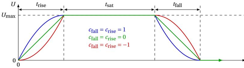
Figure 8.3: The commanded voltage profile that is used for stance phase optimisations is fully defined by the following 6 parameters: the maximum supply voltage  $U_{\max}$ , the durations  $t_{\text{rise}}$ ,  $t_{\text{sat}}$  and  $t_{\text{fall}}$  and the curvature parameters  $c_{\text{rise}}$  and  $c_{\text{fall}}$ . The different colours show the effect of different values for curvature parameters.
