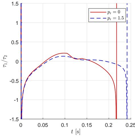
(a) The GRF is shown to be within a  $90^\circ$  friction cone ( $|\tau_1/\tau_2| < 1$ ), except shortly after landing and shortly before take-off.
