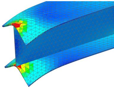
Figure 6.8: Bending illustrated of a vertically loaded thin I-beam ( $D/t = 40$ ), which shows the top and bottom open end plates turning away and taking less stress: effectively losing their effectiveness.
