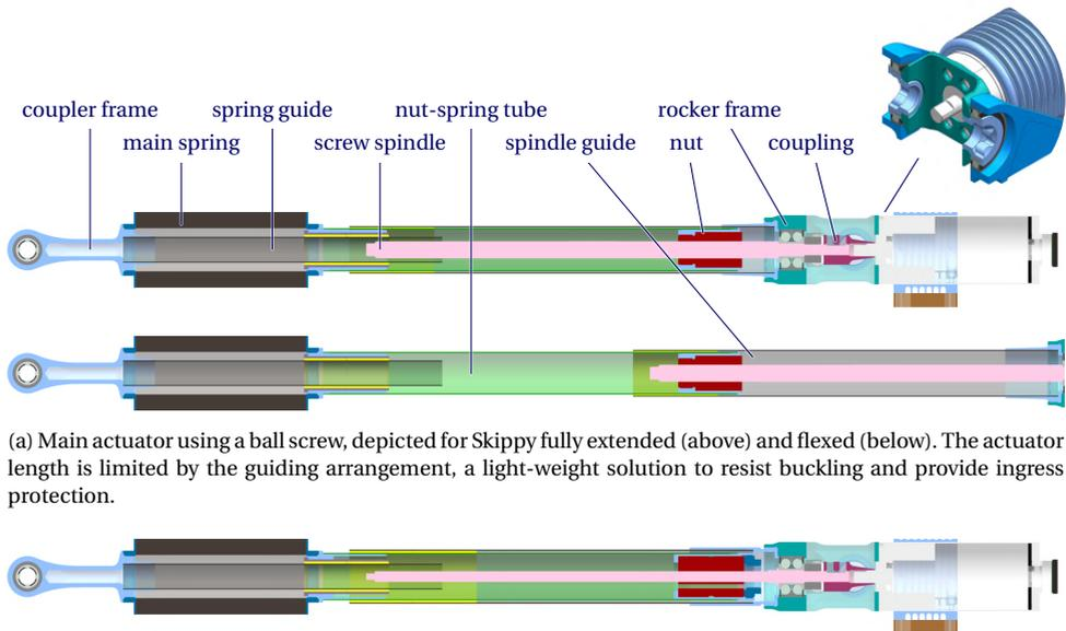
(a) Main actuator using a ball screw, depicted for Skippy fully extended (above) and flexed (below). The actuator length is limited by the guiding arrangement, a light-weight solution to resist buckling and provide ingress protection.
