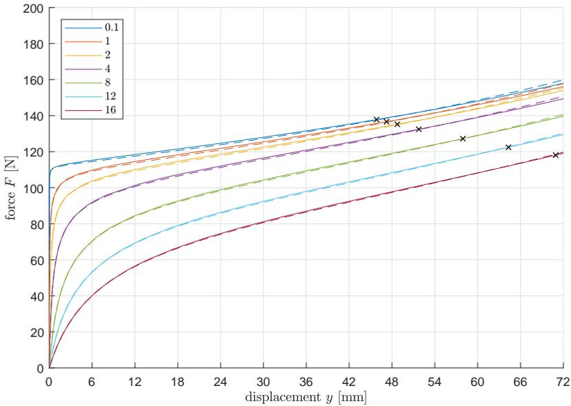
Figure 7.3: Spring profile: force  $F$  versus displacement  $y$  according to FEAs (solid) and algebra (dashed) for various arc widths  $a$  (see legend). Parameters:  $k_c = \pi^2/4$ ,  $\lambda = 0.6$ ,  $L = 144$  mm,  $I = 6.75$  mm<sup>4</sup>,  $E = 35$  GPa. Black x-marks correspond to a maximum compressive strain of  $\epsilon_{xc} = 0.21$  according to FEAs, which is assumed to be the compressive strain at which material failure is imminent (see also fig. 7.6).
