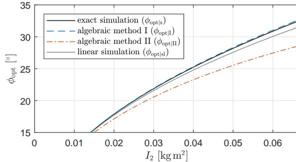
Figure 4.3: Results of algebraic method I ( $\phi_{\text{opt|I}}$ ) match very well with those of the exact simulations ( $\phi_{\text{opt|s}}$ ) and slightly poorer—but still well—with those of simulations with a linearised component of the gravity force ( $\phi_{\text{opt|sl}}$ ). Results of algebraic method II ( $\phi_{\text{opt|II}}$ ) match much poorer with both  $\phi_{\text{opt|s}}$  and  $\phi_{\text{opt|sl}}$ .
