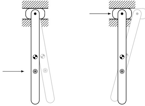
Figure 6.20: A slender beam suspended from a pivot on a frictionless slider, with the CoM (●) at  $c_x = 1/2l$  and the CoPc (⊗) at  $p_x = 2/3l$  from the pivot point. The initial response is shown in grey: if struck by an impact at the CoPc (left), then no initial displacement occurs at the pivot, and the other way round (right).
