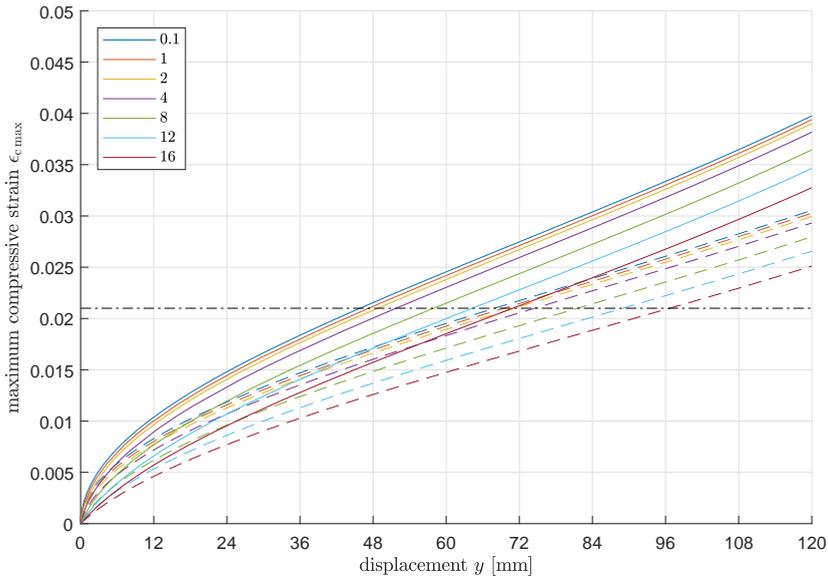
Figure 7.5: Maximum compressive strains corresponding to data in fig. 7.3, with strains according to eq. (7.13) with  $M_b = M$  and  $F_n = F$  dashed. The fit is poor. The failure compressive strain  $\epsilon_{c,c} = 0.021$  is plotted dash-dotted in black.
