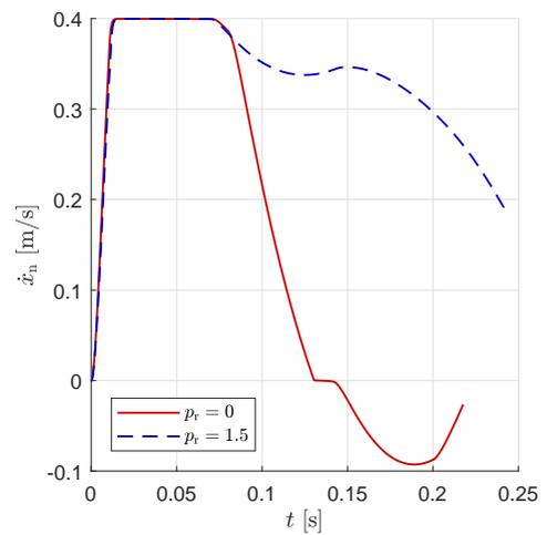
(d) Nut velocity  $\dot{x}_n$ , causing the input voltage  $U$  to be saturated so as to not exceed the maximum permissible speed of  $0.4 \text{ m s}^{-1}$ .
