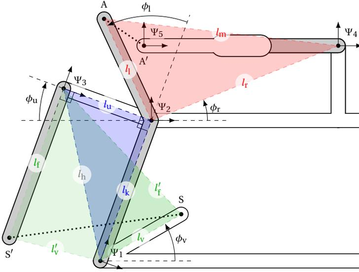
Figure C.1: Full kinematic model of Skippy's hip joint in its zero position ( $q = \mathbf{0}$ ). The loop closure constraints are not satisfied. Not to scale.
