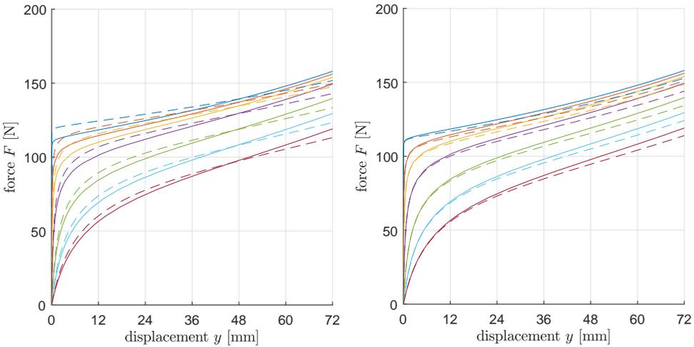
(a)  $\lambda = 0.85$ ,  $k_c = 2.65$ (b)  $\lambda = 2/3$ ,  $k_c = \pi^2/4$ Figure 7.4: Results for different values of  $\lambda$  and  $k_c$ .
