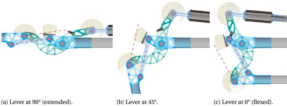
Figure 6.14: Skippy's hip range. The distance between the red dashed lines is the moment arm of the follower  $a_f$ . When Skippy is fully flexed (more torque)  $a_f = a_{f, \text{flx}} = 5 \text{ cm}$  and when it is fully extended (more speed)  $a_f = a_{f, \text{ext}} = 2 \text{ cm}$ .
