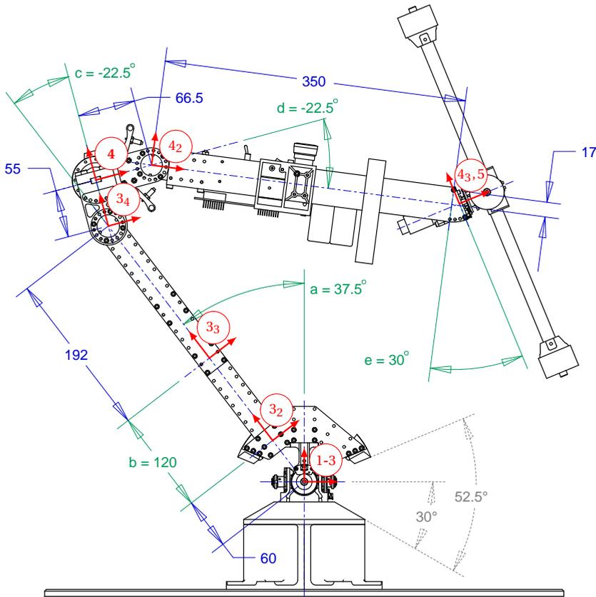
Figure 5.3: Right view of Tippy, scale 1:6.25. Fixed dimensions displayed in blue and tunable dimensions in green with parameters  $a$  to  $e$ , with lengths in mm and angles in  $^\circ$ . All joint angles are zero ( $q = 0$ ). Right-handed  $yz$  coordinate frames of (sub-)bodies in red, with  $x$  pointing out of the drawing.
