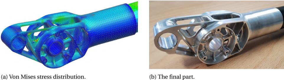
Figure 6.12: Images depicting the lower end piece of the torso's frame, with left an image showing stress distributions of the FEA corresponding to the load case depicted in fig. 6.11 and right the machined part.
