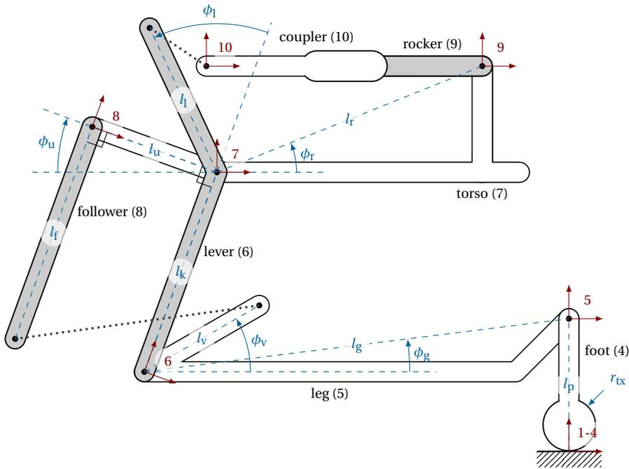
Figure 8.1: Full kinematic model of Skippy in its *open-loop zero* configuration  $\mathbf{q} = \mathbf{0}$ , not to scale. Loop closure constraints would be satisfied if the points connected by the two dotted lines coincided, forming revolute joints. Joint coordinate frames and corresponding joint numbers are drawn in red; body names and corresponding numbers are written in black. Their transformations and loop closure kinematics are fully defined by the 14 indicated parameters.
